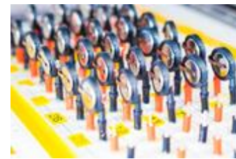
Next-generation lithium-sulfur battery under charge/discharge performance evaluation
