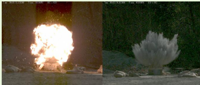
Difference in explosion with and without the power reduction agent (left: without the agent; right: with the agent (almost no flame)) Provided by the Explosion Investigation Section, Second Department of Forensic Science, National Research Institute of Police Science
