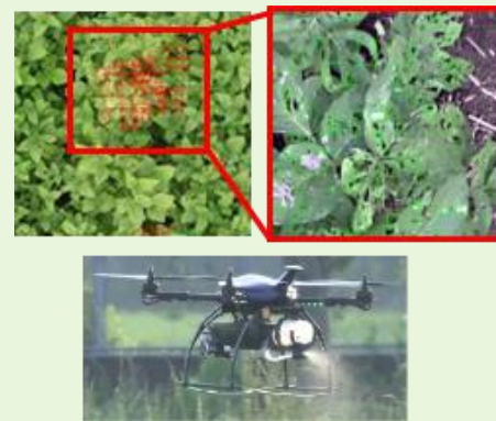
Detection of pest damaged parts by AI (above) Pinpoint chemical spraying by drone (below) Provided by OPTiM Corp.
