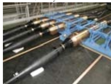
Seabed observation cable network (Seismometers and water pressure meters) Courtesy of MEXT
