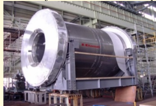
Liquid argon vacuum chamber Kawasaki Heavy Industries, Ltd.
