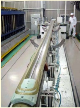
Beam-converging superconductive quadruple magnet Source: Toshiba Power Systems Company
