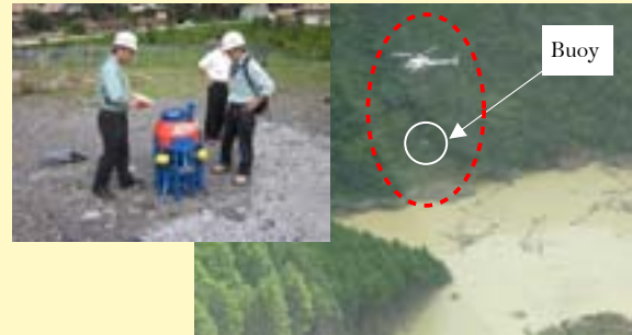
Appearance and setting condition of PWRI's aerielly placeable floating water gauge Courtesy of Ministry of Land, Infrastructure, Transport and Tourism, Kinki Regional Development Bureau
