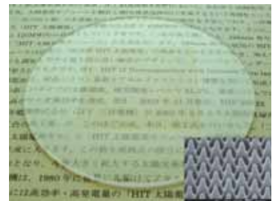
anti-reflection structured surface (patterned part 50mm x 50mm: SANYO Electric Co., Ltd.)
