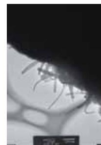
TEM photo of carbon nanotube
