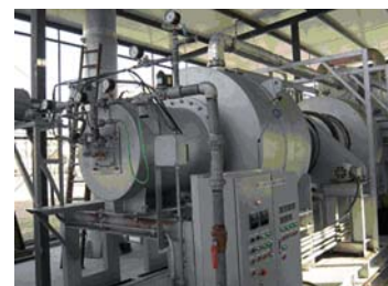
Equipment required for reduction and heat treatment (experimental site at Shanghai Jiao Tong University)
