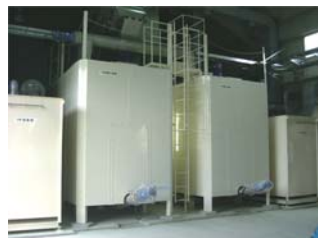
Ex. 3. Fermentative treatment unit for organic sludge, as developed by Mishima Co., Ltd
