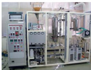
Test setup for the gasification of woody biomass
