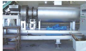
Equipment required for the waste carbonization (reduction and heat treatment) process (rotary kiln)
