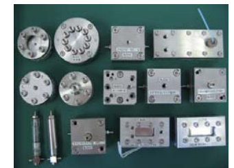
Example of micro-reactor
