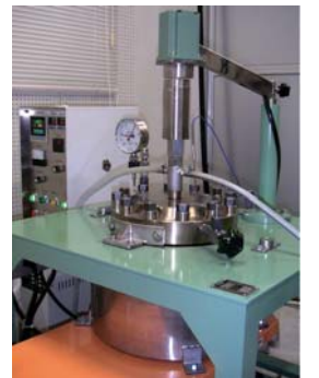
Environmental simulation testing machine that simulates the environment of an actual machine with high temperatures and pressures
