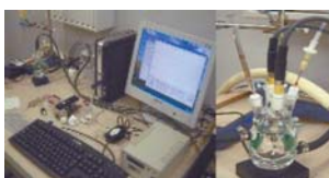
Gas sensor using a molecular recognition compound
