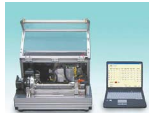
Prototype machine for the internal finishing of tubes
