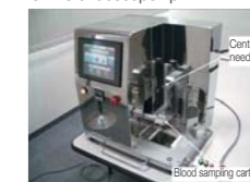
Prototype of in-vivo analyzer that uses micro-samples
